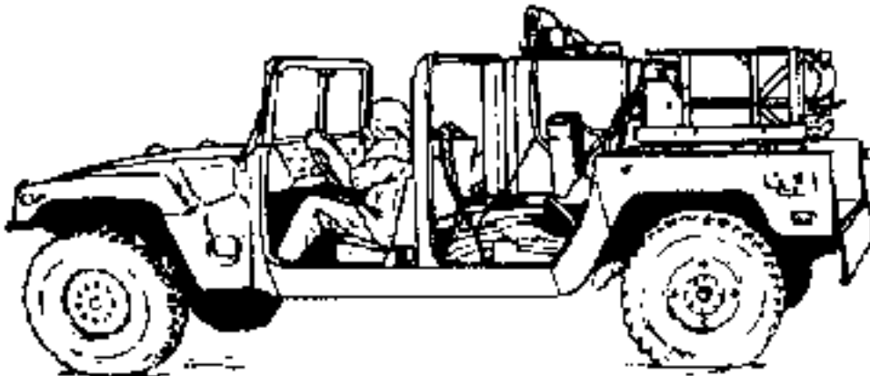
Figure A-III-4. Motorized smoke system.
